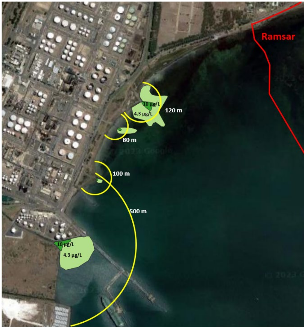
Figure 3-5. Inferred Chlorine Contours in Existing Plumes
