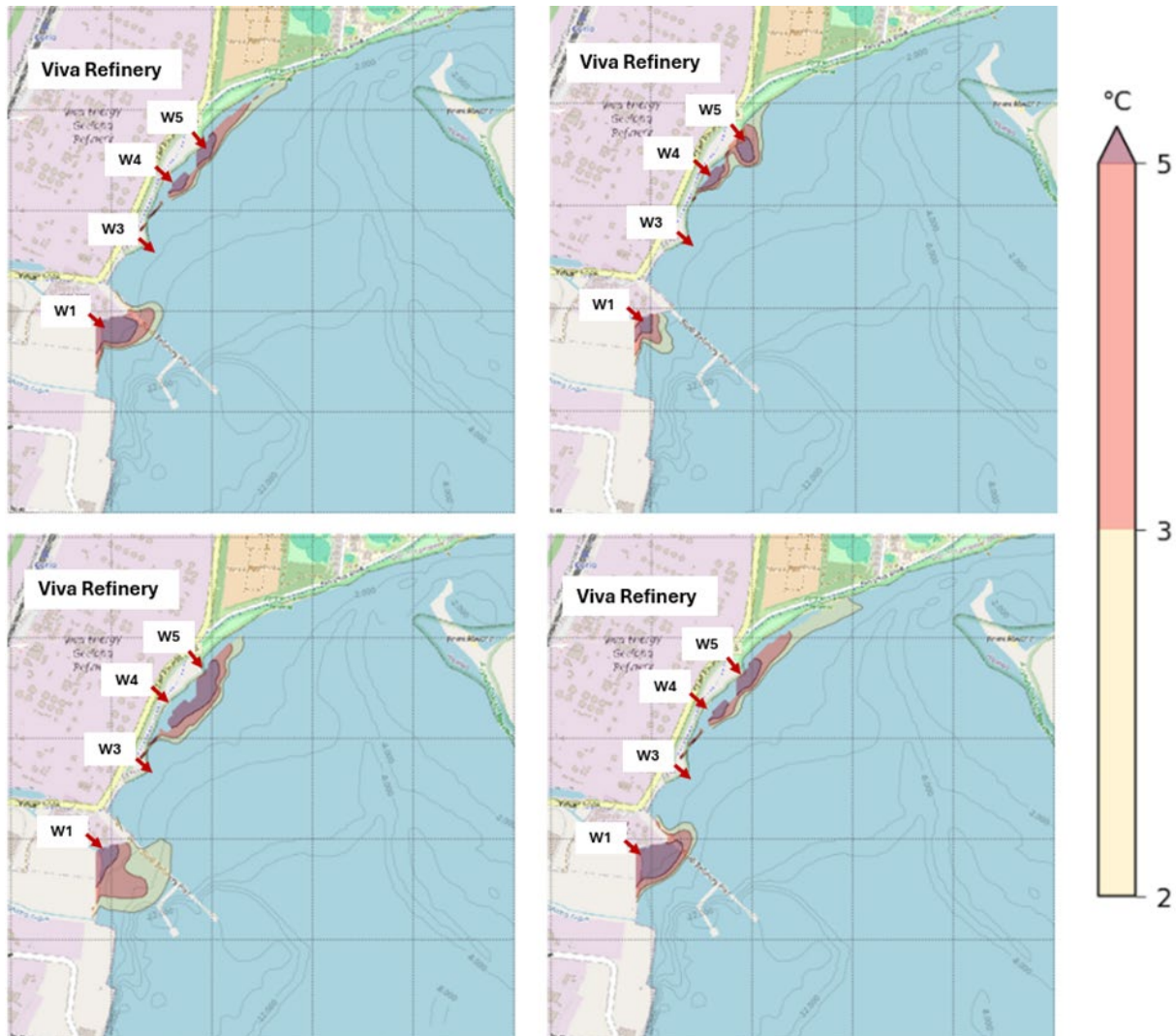
Figure 4-8 Predicted temperature plumes using the refined regional hydrodynamic model
