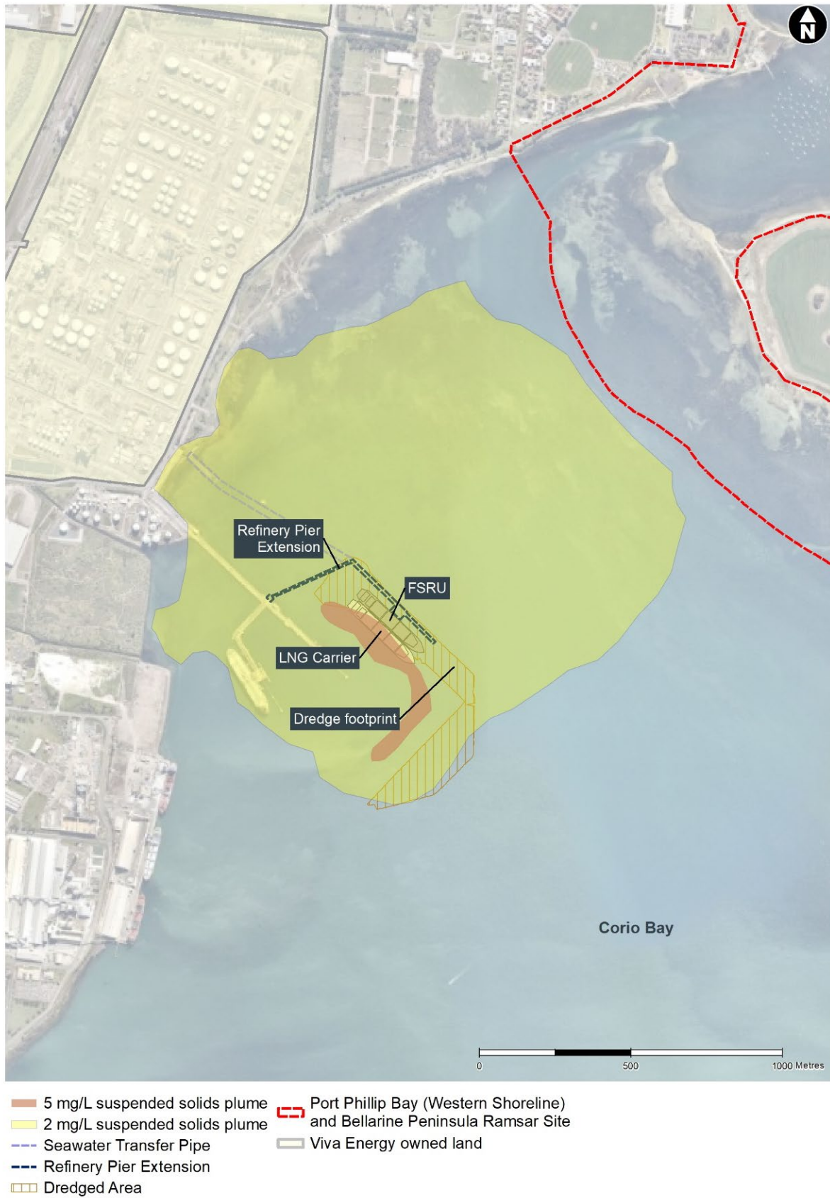
Figure 4-2 Average increase in suspended solids concentration above ambient at surface during dredging
