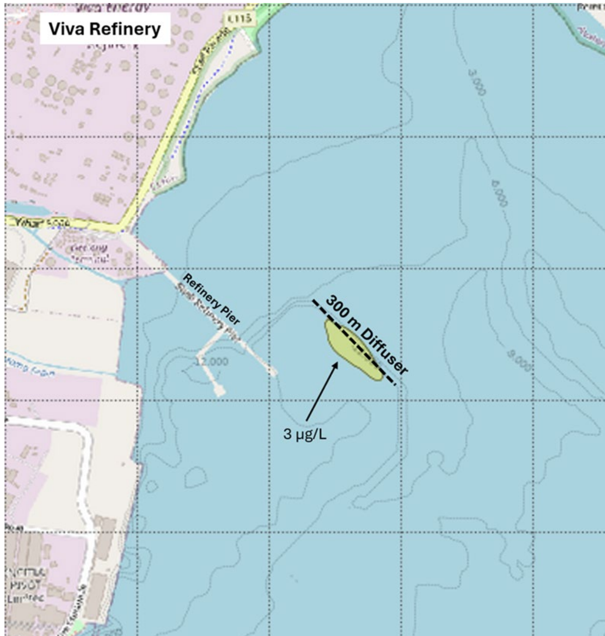
Figure 4-11 Predicted chlorine plume – FSRU discharge through the diffuser
