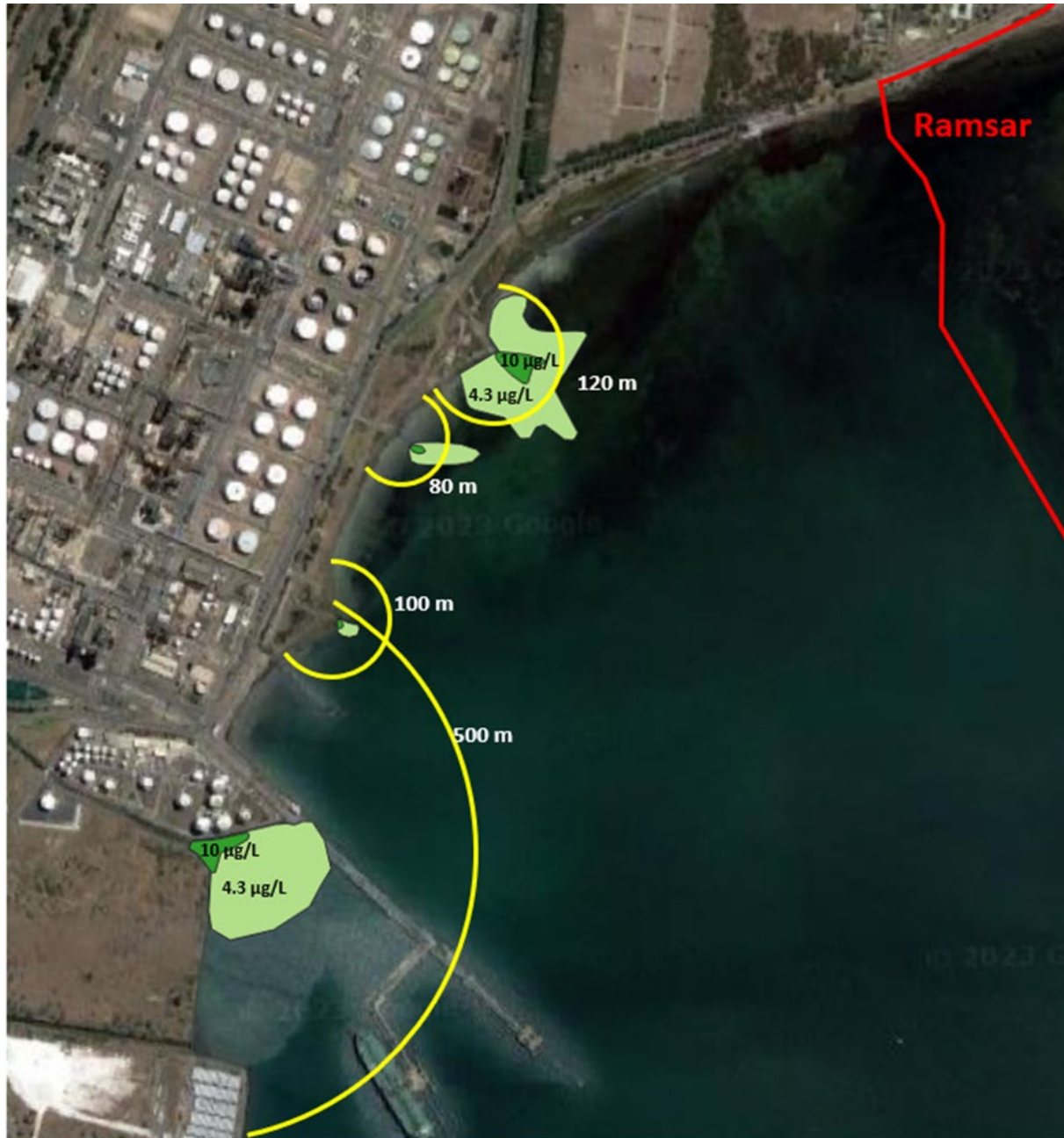
Figure 4-9 Inferred chlorine contours in existing plumes.
