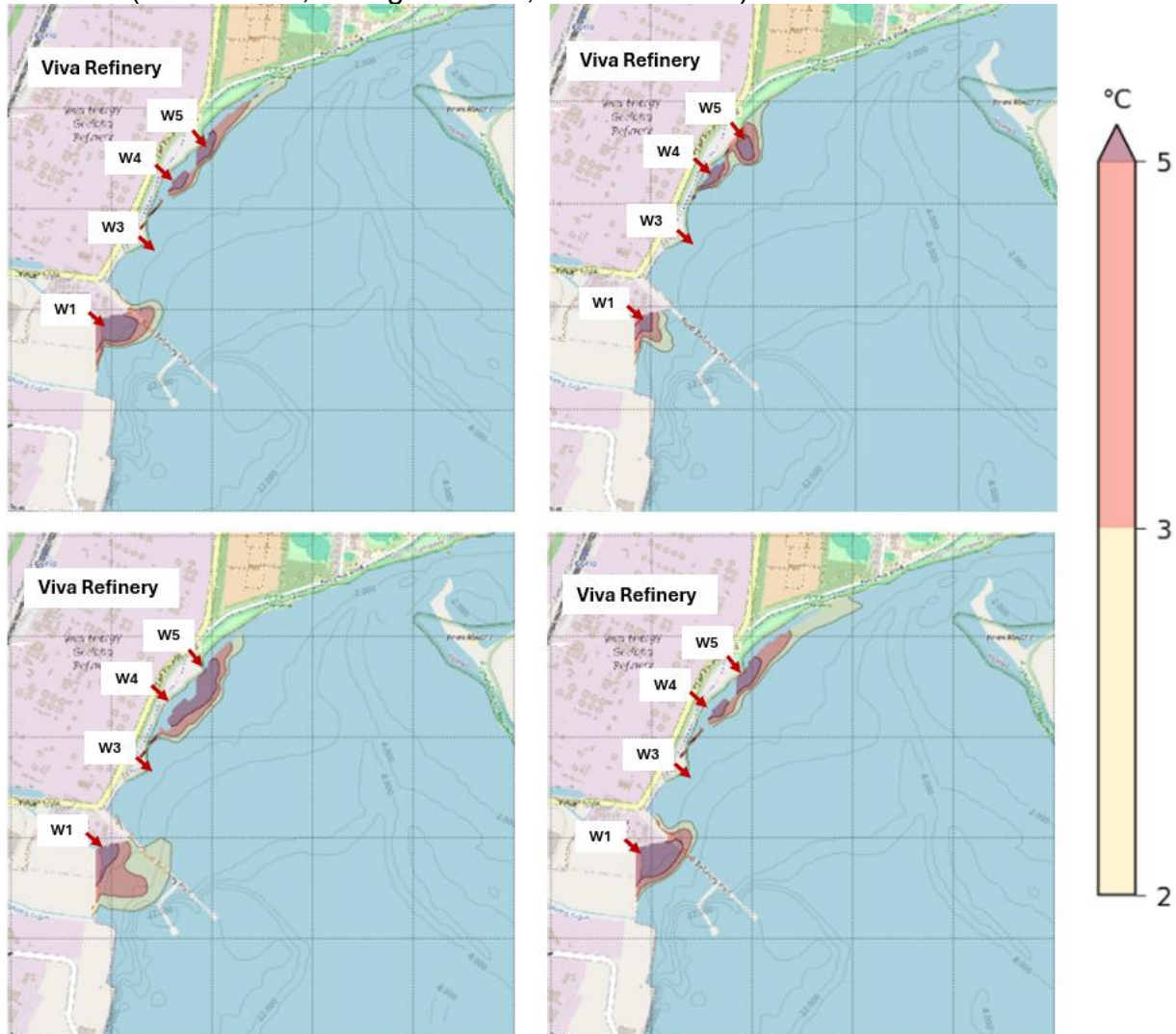
Figure 1-1. Predicted Temperature Plumes Using Refined Model
