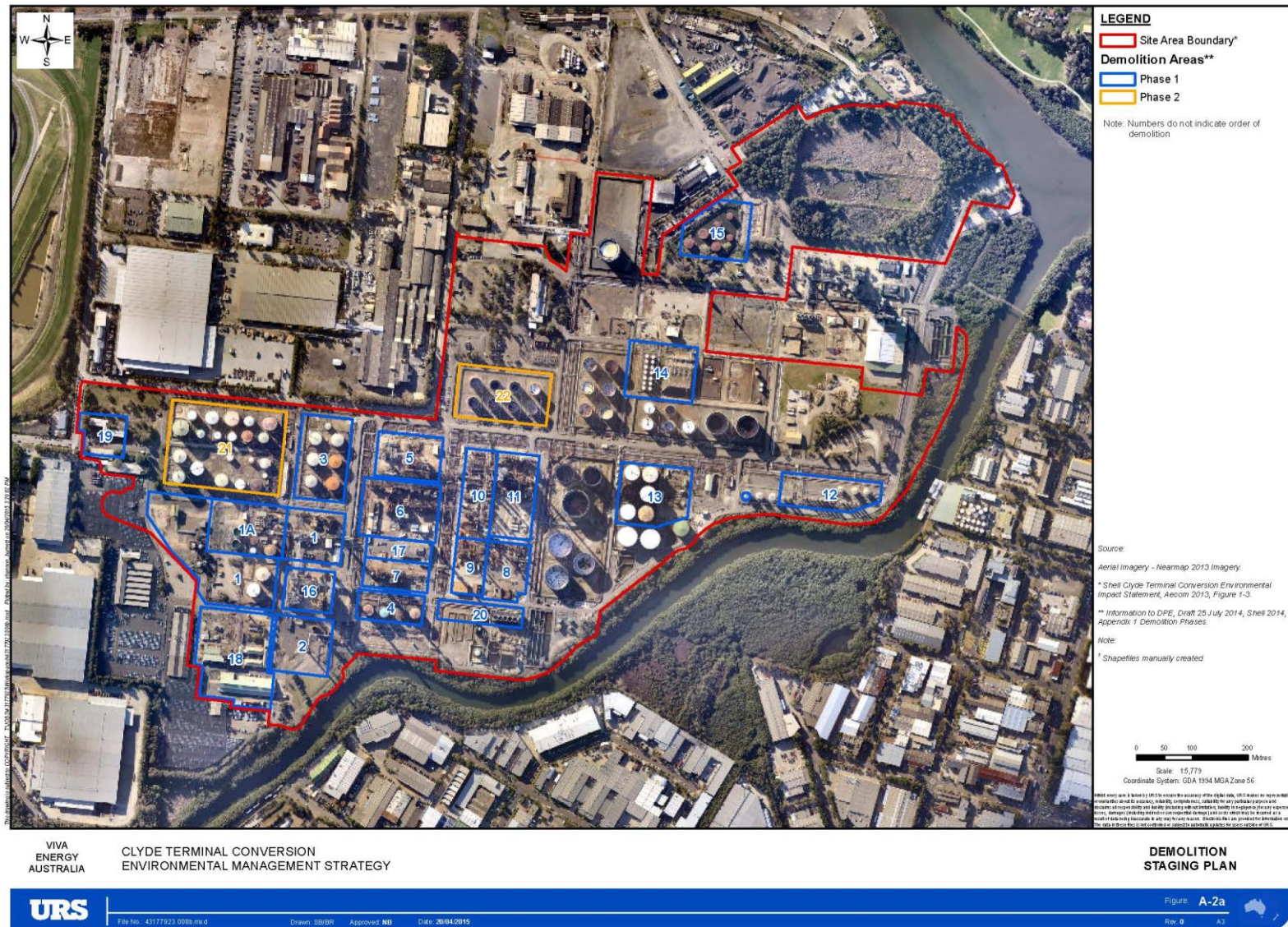
A.1 Figure A.1 Demolition staging plan
