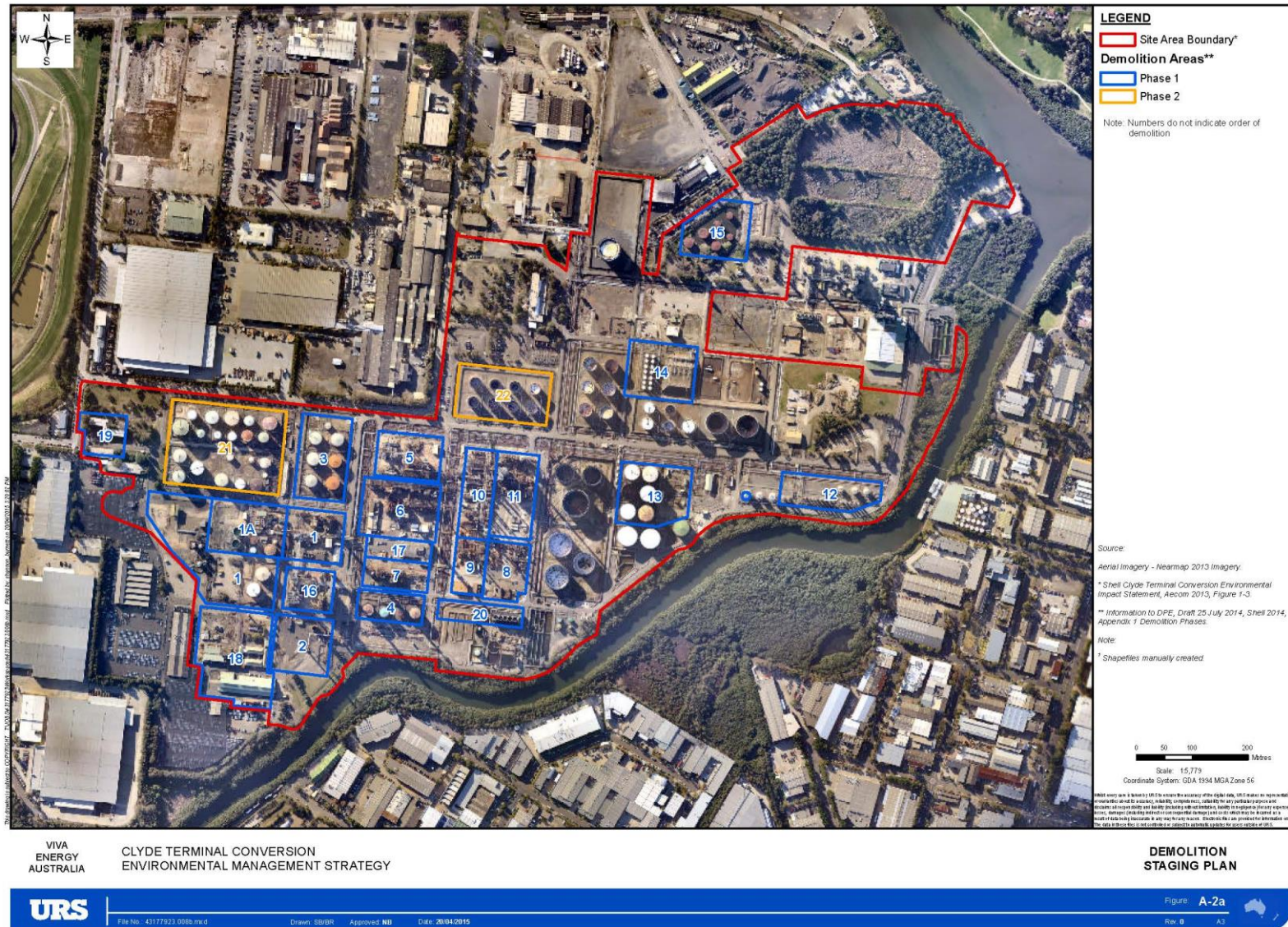
A.1 Figure A.1 Demolition staging plan
