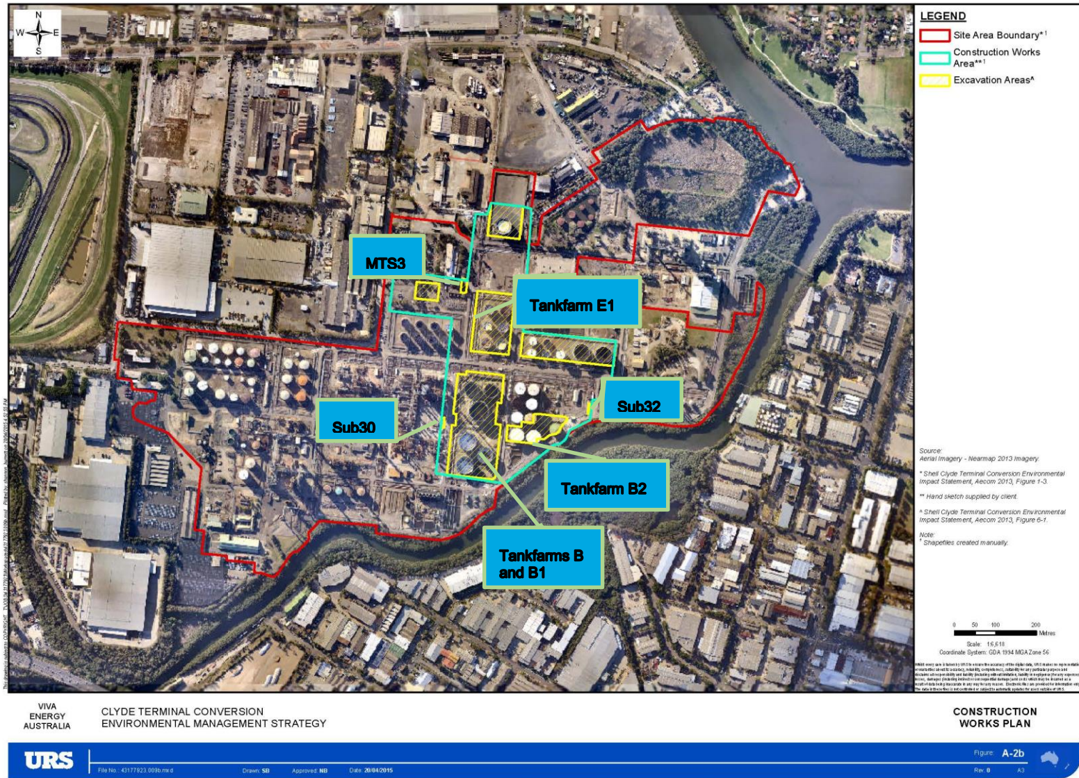
A.2 Figure A.2 Construction works plan
